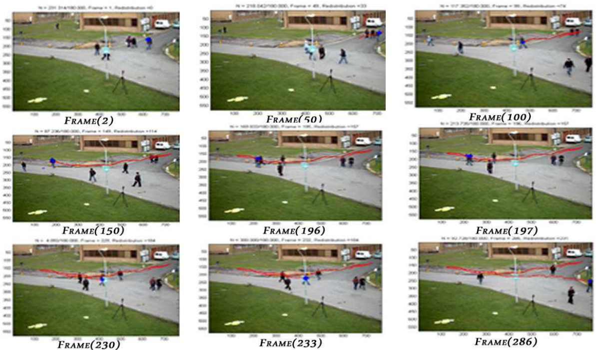
Figure 6 Tracking result for outdoor dataset using 300 particles.
